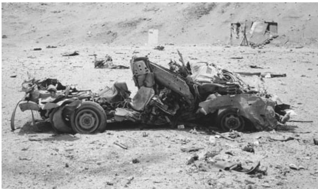
FIG. 15— Photograph of a vehicle placed at 15 m from a 2268 kg LAN/S charge.
