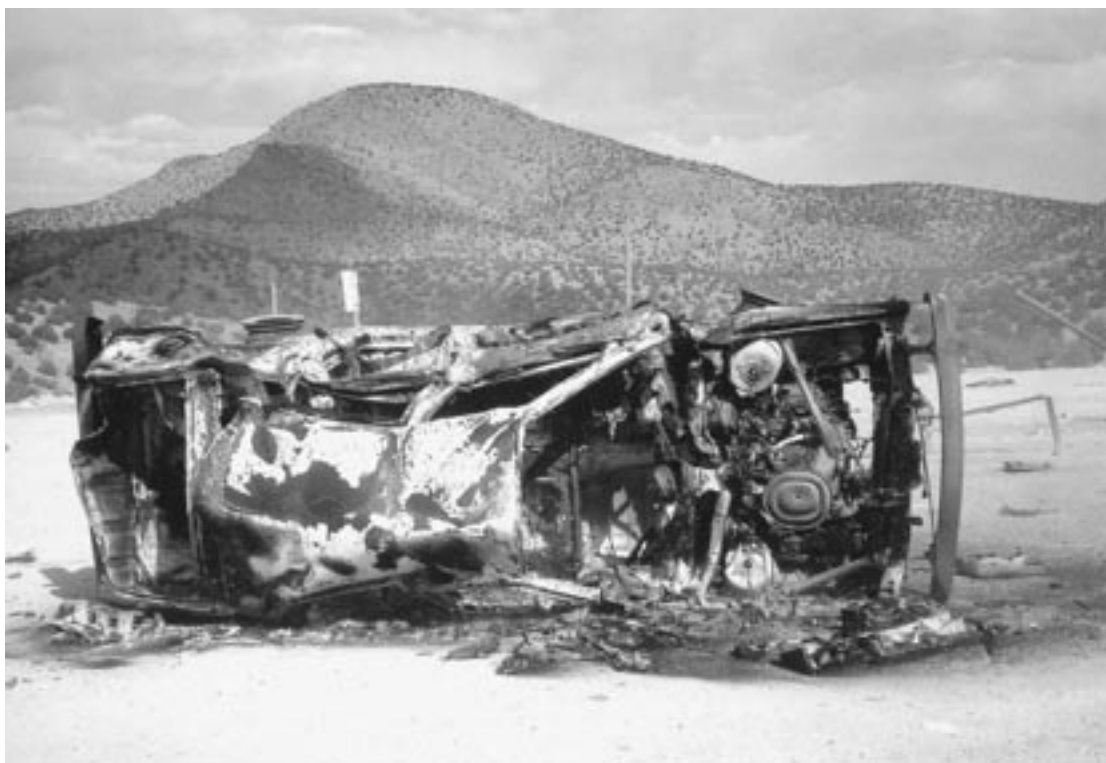
FIG. 12—Photograph of a vehicle placed at 15 m from a 454 kg TNT charge.
