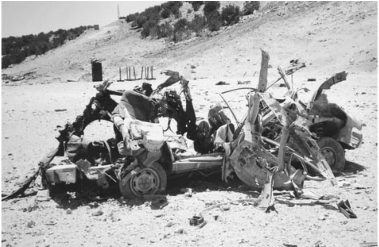
FIG. 13— Photograph of a vehicle placed at 15 m from a 2268 kg ANFO charge.
