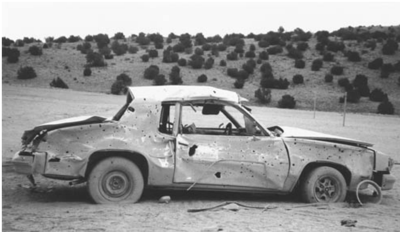
FIG. 14— Photograph of a vehicle placed at 15 m from a 454 kg LAN/S charge.
